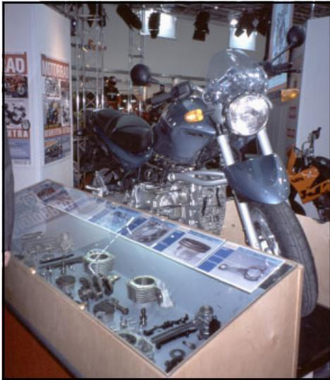
Motorrad had tested one for 30,000 miles and then disassembled it to find if there was any wear. The only wear they found was at the plastic timing chain tensioner.
