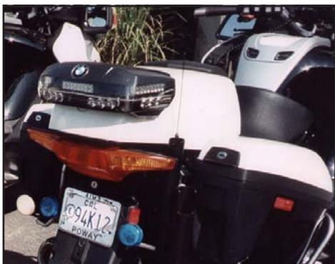
The rear view shows that the famous bubble gum flashing lights are no more. They are replaced by banks of LED's.
